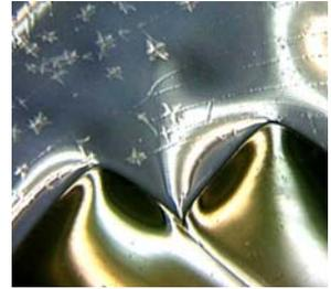
Cracks and splits after fusing.
