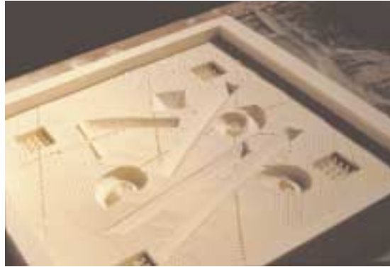
Dry plaster mold ready to fill with glass
