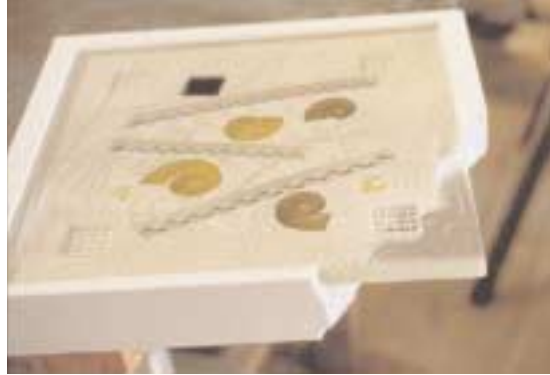
Mold material carefully broken away from the glass casting
