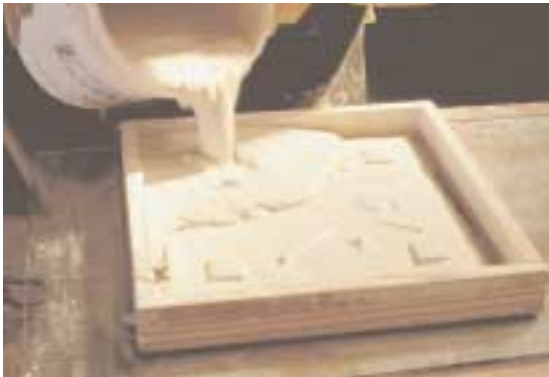
Over fill mold box slightly
