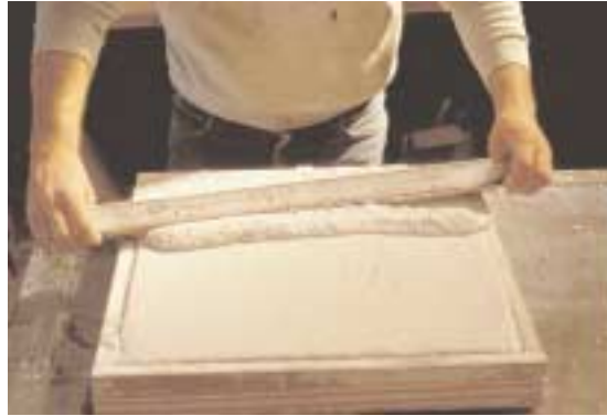
Excess plaster screed off
