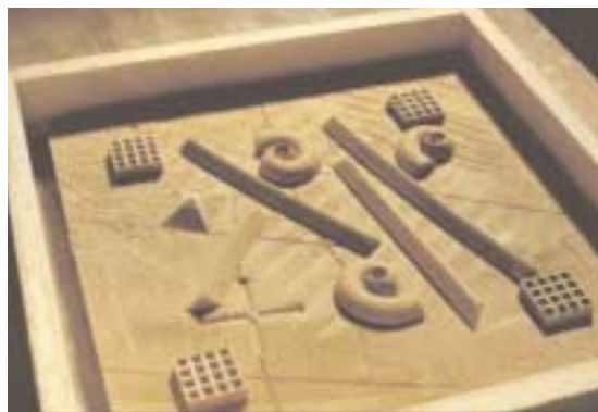
Mold boards used around clay positive
