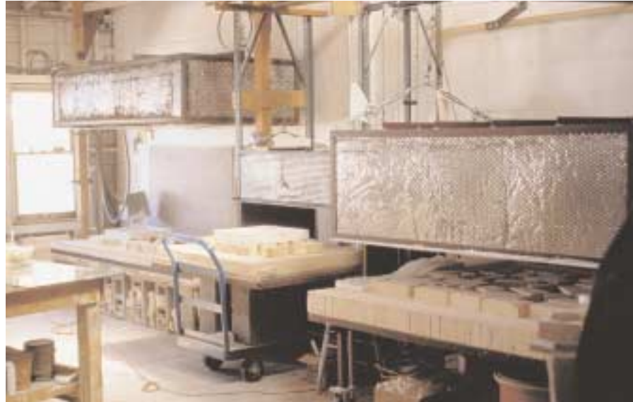
Fired glass mold coming out of the kiln
