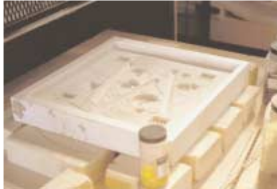
Various frit sizes and colors added to mold cavities
