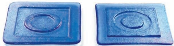
Figure 3d: Glass after firing, kilncarved side up.
