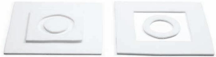
Figure 3a: Positive and negative ceramic fiber paper designs.
